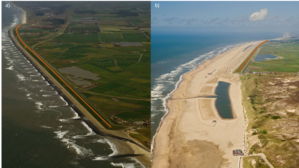
Figure 2.1.: a) Hondsbossche sea dike before placement of the nourishment (courtesy of Rijkswaterstaat, https://beeldbank.rws.nl/ , accessed on 6 September 2021) and b) the Hondsbossche Dunes Nourishment just after placement in April 2015 (courtesy of Annemerscombinatie Zwakke Schakel–Van Oord-Boskalis). The orange line marks the crest of the original sea dike.
