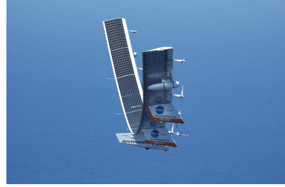
(b) Helios at high wing dihedral prior to structural failure and in-flight breakup, ©NASA
