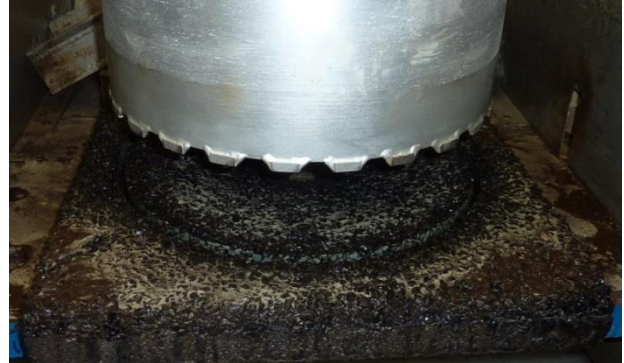
Figure 12: Coring of asphalt sample with a diameter of 390 mm
