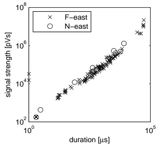
Figure 9. Duration vs. Signal strength of AE hits generated by walking above the bridge deck.
