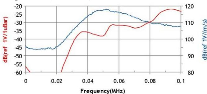
Figure 5. Transfer function of R6I-AST (Physical Acoustics, 2016).
