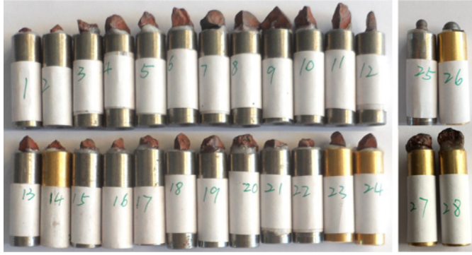
Figure 4.9: Experimental pins with SiShen particles
