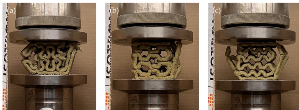
Figure 7. Compression test: (a) curved; (b) honeycomb; (c) rhombic.
