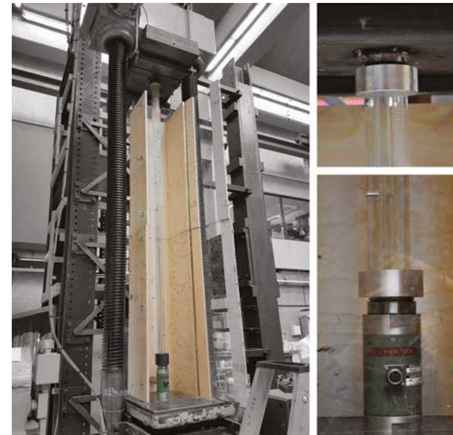
Fig.11: Left: Experimental set-up of one of the specimens. Right: Top and bottom pinned connections of the experimental set-up.
