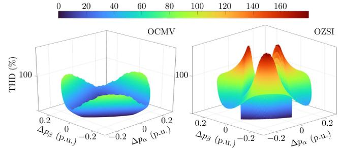
Fig. 7. THDs of the OCMV and the common-mode voltage proposed by [11] (OZSI).
