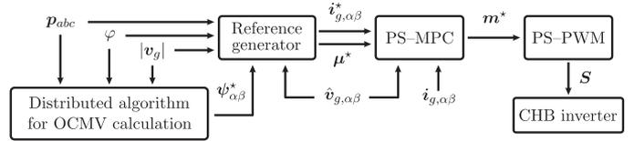
Fig. 5. Overall control scheme.
