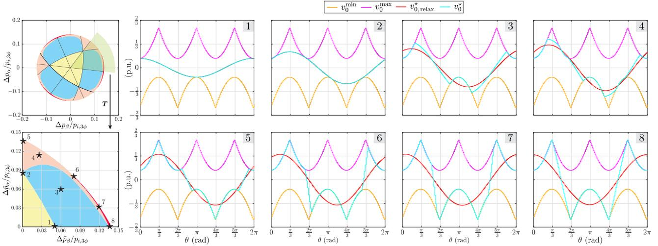
Fig. 6. First column: Feasible domain  $\mathcal{O}$  (up) and transformed sextant with analyzed points (down). From the second to fifth column: Sampled waveform of the common-mode voltage max/min limits, relaxed solution, and the OCMV.
