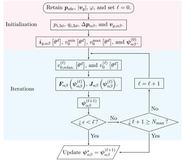
Fig. 3. Flowchart of the distributed algorithm for the OCMV's iterative calculation.
