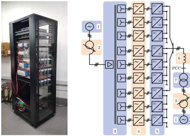
Fig. 9. Test bed and its unilinear diagram. Glossary: 1) Grid. 2) Variable autotransformer. 3) Multiwinding transformer. 4) Three-phase diode rectifiers. 5) HBs. 6)  $L$  filter. 7) Isolation transformer.
