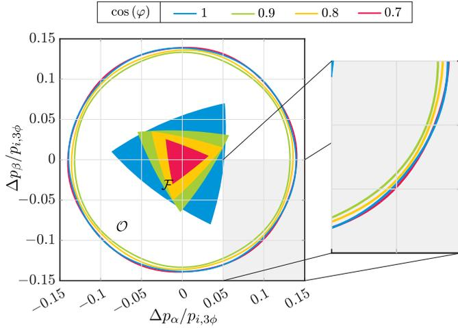
Fig. 2. Feasible domain  $\mathcal{O}$  and feasible domains  $\mathcal{F}$  for various power factors  $\cos(\varphi)$  considering  $\frac{p_{i,3\phi}}{3} = \frac{2}{3}$  p.u.
