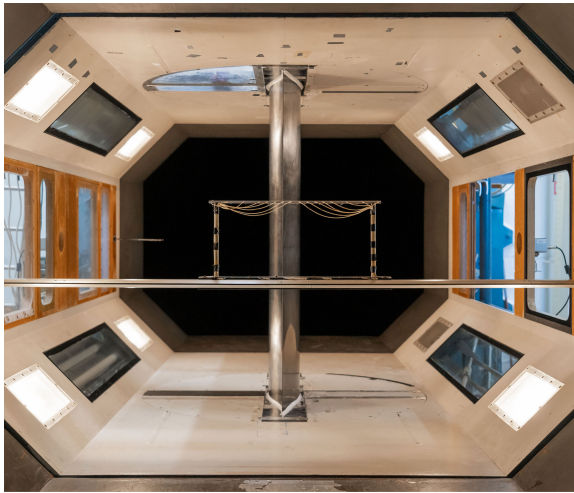
Figure 2. The octagonal LTT testing section with the wake rake and the airfoil model set to AoA = 0^\circ . View from downstream of the trailing edge.
