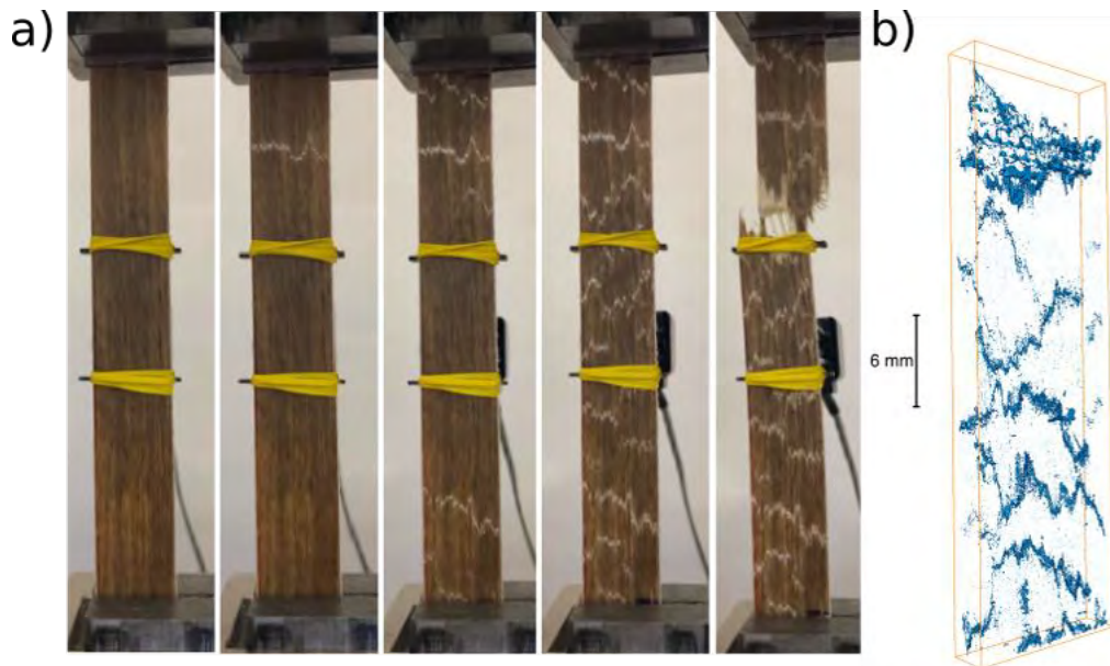
Figure 3. a) Visual development of the fragmentation process and b) internal image using XCT observation of the damage mechanism which resulted in the appearance of pseudo-ductile behaviour,
