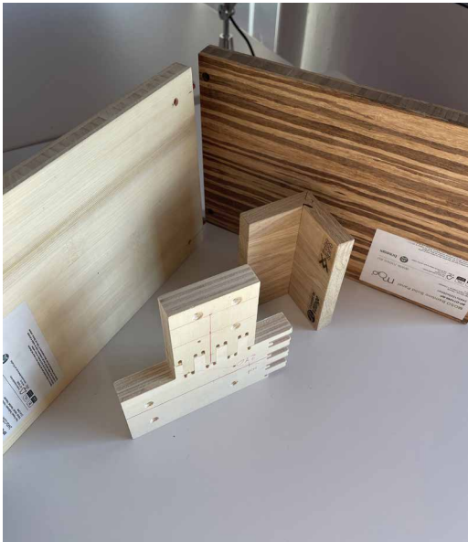
FIG. APP.C.4 Multiple mock-ups of types of connections for the CIK frame
