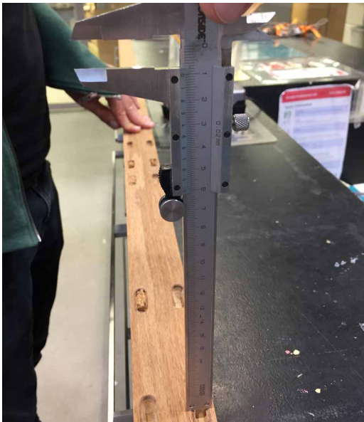
FIG. APP.C.6 Measuring depth in a mock-up for the tool-free click-on connector in bamboo
