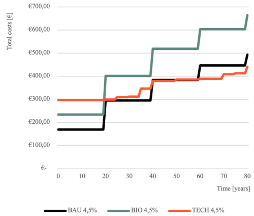
FIG. APP.A.4 LCC Sensitivity analysis on the influence of interest rate when comparing kitchen variants (baseline, scenario 1)
