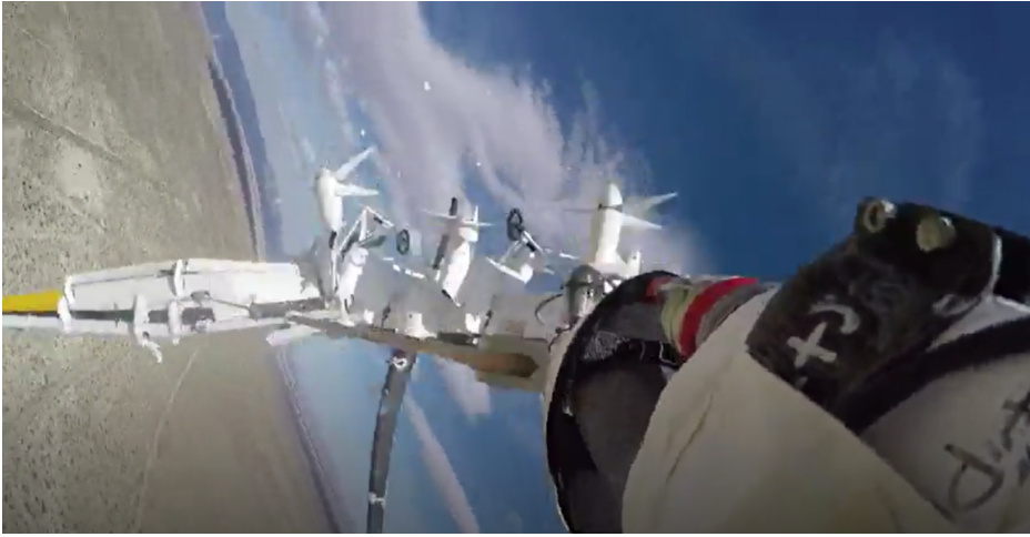
Figure B.6: Mid-Air Break Up of Makani M600 During Crosswind Flight [150].
