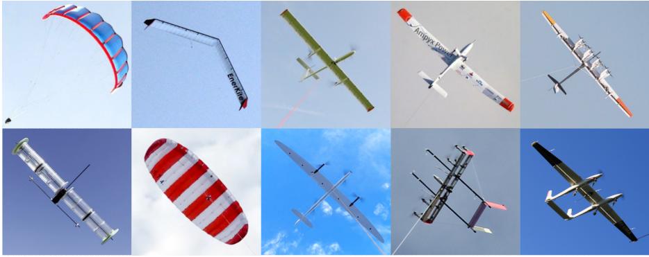
Figure 1.1: Selected AWES concepts: Kitepower, EnerKite, TwingTec, Ampyx Power, Makani Power, Wind-Fisher, Skysails, Kitemill, Kitecraft, Mozaero (photos from AWEC conferences book of abstracts).
