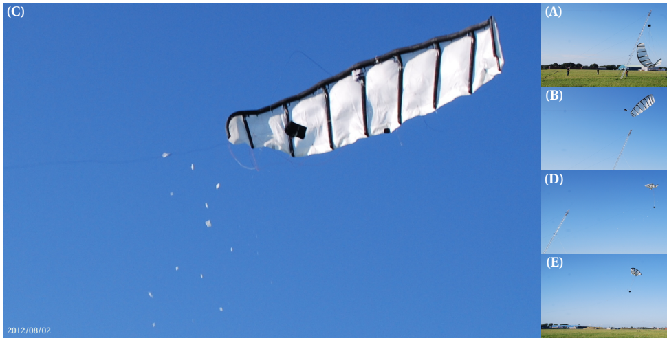
Figure B.1: Experimental mast-based launch of the LEI V3 kite (A-B), breaking weak link due to a sudden overload (C) and descent of the damaged wing while being secured by the safety line (D-E) [56].
