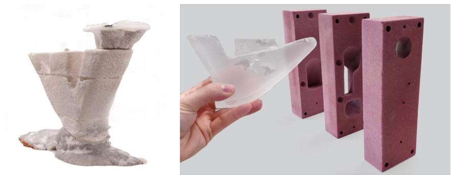
Fig. 4 left: part of TO glass column as realized in 3DPSM made of silica sand and CHP binder, right: same glass part after manual polishing and on the back segmented 3DPSM used for the casting (before firing) (Oikonomopoulou et al. 2020)
