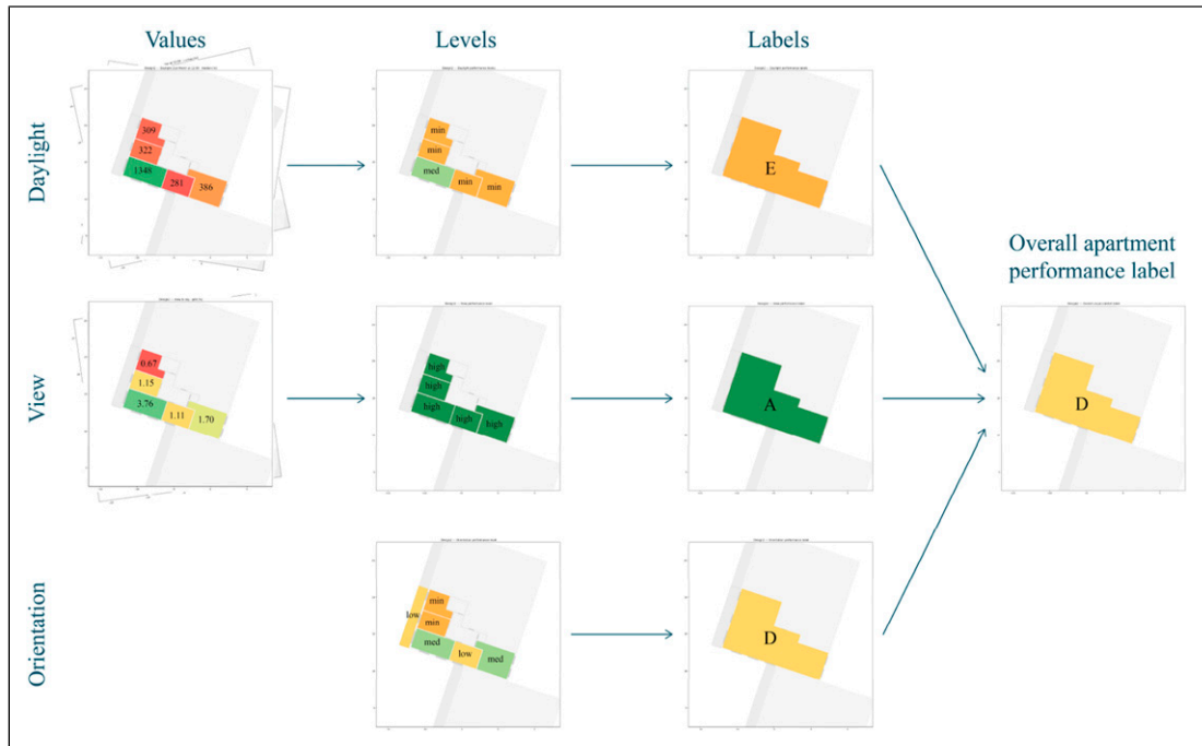
Figure 13. Example of layout evaluation system and ranking for a layout design option.
