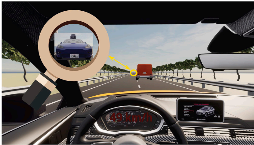
Fig. 2. Participants' perspective while performing the task in the driving simulator. The lead vehicle blocks the view of oncoming traffic. As the participant moves to the opposing lane to assess the road situation a decision has to be made to either overtake the lead vehicle (accepting the gap) or stay behind the lead vehicle until the oncoming car passes (rejecting the gap). The inset depicting an oncoming vehicle is for illustrative purposes only and was not present in participants' view during the experiment.
