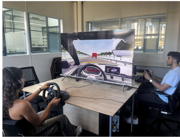
Fig. 1. “Reverse Wizard-of-Oz” experimental setup of the driving simulator. During the sessions involving oncoming “human-driven” vehicles, the experimenter (on the right-hand side) was not visible to the participant (who also could not see the movements of the experimenter’s steering wheel) and pretended to operate an unconnected driving simulator. The participant wore a noise-canceling headset to avoid hearing the experimenter’s control inputs.
