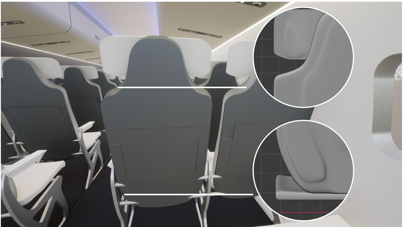
Figure 3: Highlighted cut outs in the seat.
