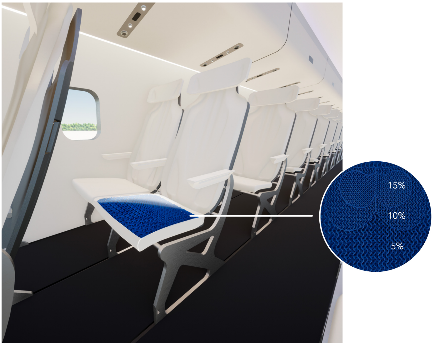
Figure 1: Seat pan with different infill percentages to support different parts of the body; this method can also be used for the backrest.
