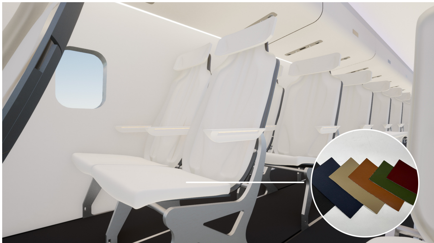
Figure 4: The top layer is made from cactus leather, grown locally in Brazil (close to the Embraer plant).
