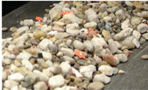
Figure 1. Material batch of natural 2-8 mm river gravel and shredded polypropylene flakes.
