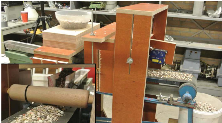
Figure 2. Conveyor setup for testing the gravel batches.
