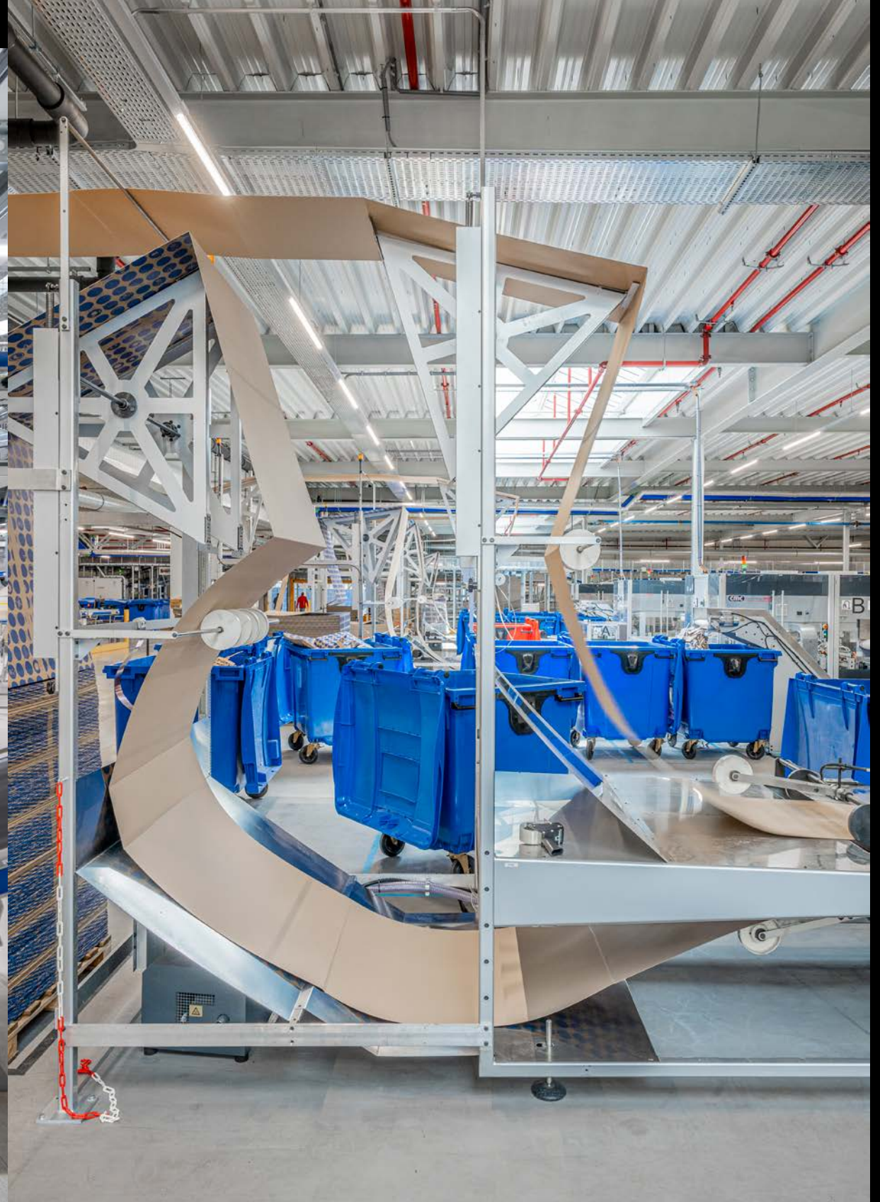
← The new generation of vertically oriented packaging system. ↑ Double carton infeed for the carton wrap package cutting machine. Each feed has a different width to reduce the carton waste.
