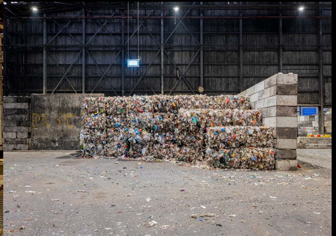
← The wind-shifter separates lightweight foil from plastic. ↑↑ Incoming waste. Sifting starts in the supply hall where waste from the acceptance area is spread with cranes and bulldozers. ↑ The semi-finished product. Approximately 1,000 bales are stored daily in the storage area before turning into raw materials or alternative fuels.
