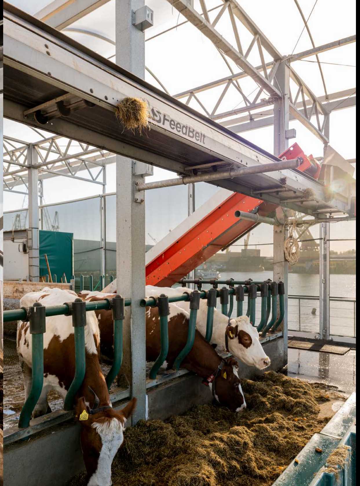
← Through the funnel, the cow's manure and urine fall from the upper-level stable into the lower-level big bags and the containers. ↑ Cows are fed three times a day through the feed-belt with residual products from the city like bread, beer broth and vegetables.
