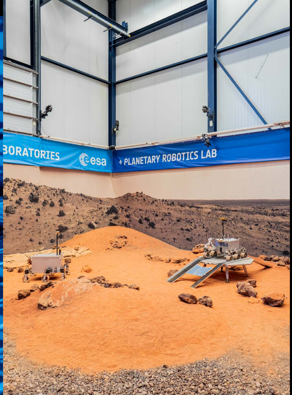
← EMC anechoic chamber. The chamber's design blocks out outside sound and absorbs acoustic echoes to simulate a space environment. ↑ A half-scale ExoMars rover is tested on terrain representing Mars's surface, which is made of sand and volcanic rocks, taken from different sites in Europe.
