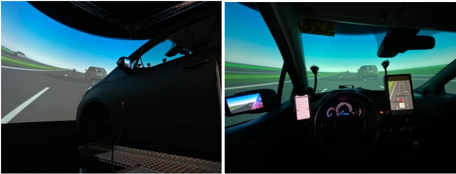
Figure 5.1: Exterior and interior of the DAVSi simulator, with visual automation UI right of the steering wheel and tablet for the questionnaire left of the steering wheel
