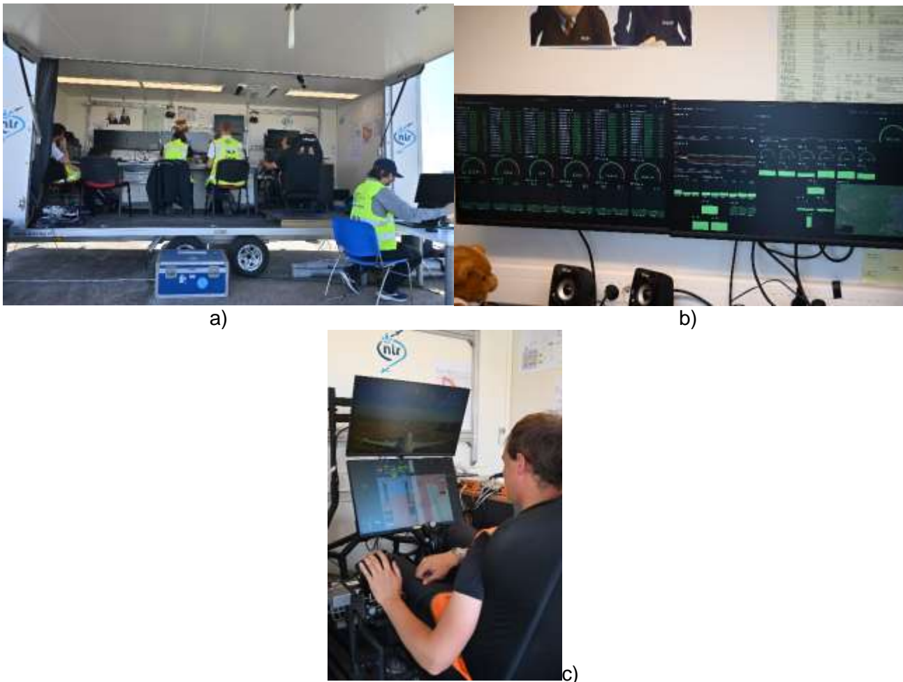
Figure 11 - The Ground Control Station from where the aircraft is BVLOS controlled and systems are monitored. a) overview of the positions for the pilot and system engineers, b) the screen on which the battery parameters (left) and FTI (right) are displayed c) pilot position
