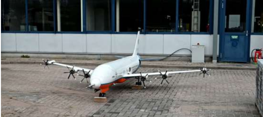
Figure 7 - DEP-SFD installed for stationary ground tests
