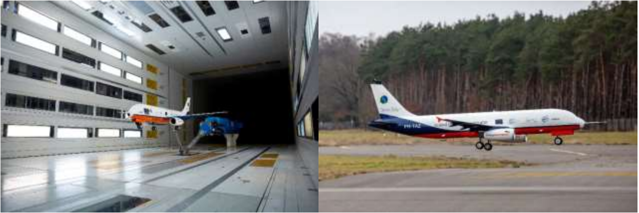
Figure 2 - SFD for the validation of the scaled flight testing methodology in the wind tunnel and in flight
