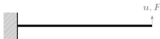
Fig. 2 Schematic of a cantilever beam under load
