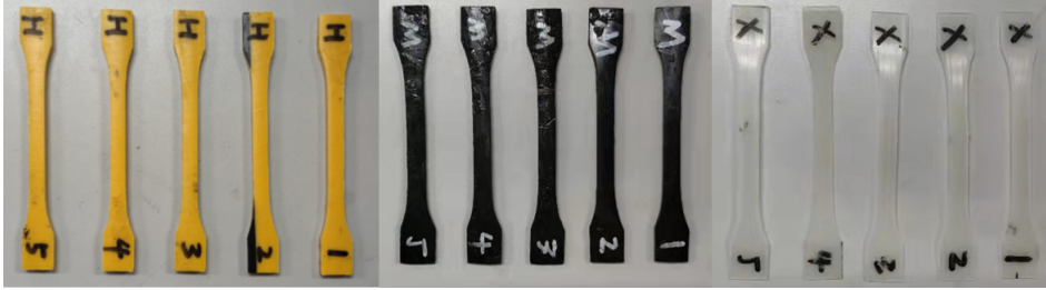
Figure 4.4: Dumbbell shape of HDPE (left), MDPE (middle) & XLPE (right)
