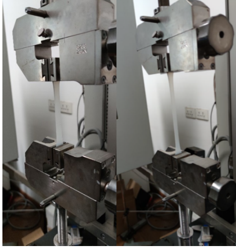
Figure 4.5: Tension test under an electronic universal testing machine
