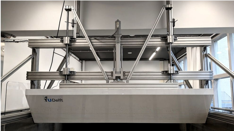
Figure 2.4: Wavemaker that generates waves at the start of the test section
