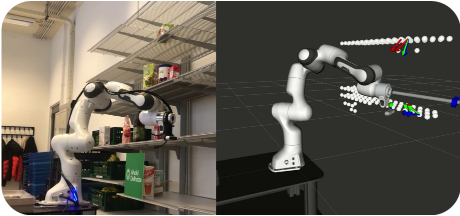
Figure 7.12: Real robotic manipulator used to run the experiments. A Franka Emika Panda is confronted with an unknown shelf environment in a supermarket. Arrows indicate the normals of the planes obtained by the FSD. Different colors indicate different links on the robotic arm.
