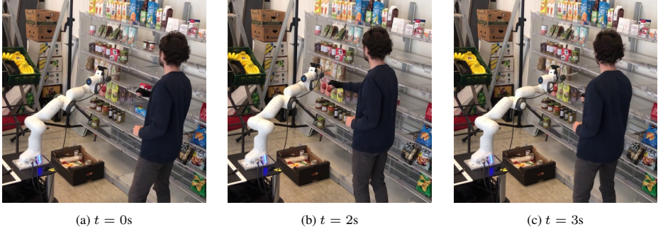
Figure 5.4: Dynamic Fabrics in the presence of a human. The human hand's state is estimated with a motion capture system. The robot smoothly and in advance avoids the human operator and allows for safe coexistence.
