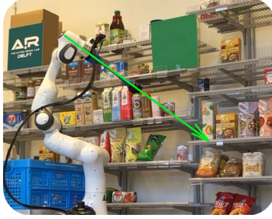
Figure 8.9: Illustration of the orientation constraints for trajectory generation for look-for-product.
