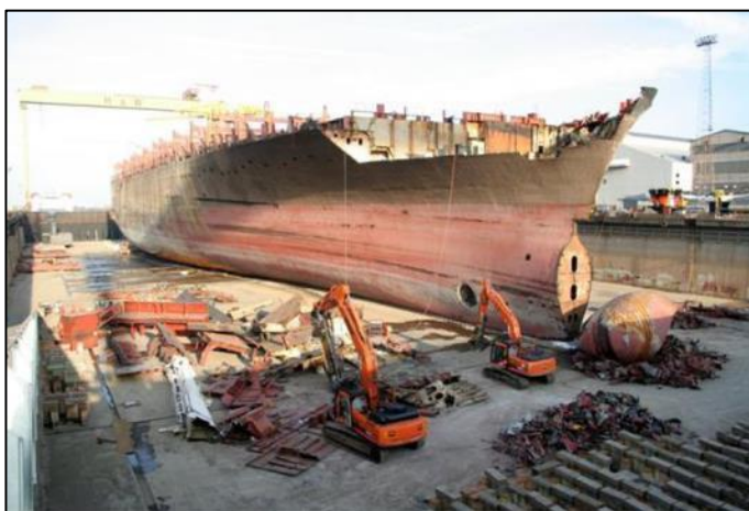
Figure 2.9: Ship dismantling in drydock (Source: www.harland-wolff.com , Image reproduced with permission of Harland and Wolff Heavy Industries Ltd., Belfast, Northern Ireland, UK)
