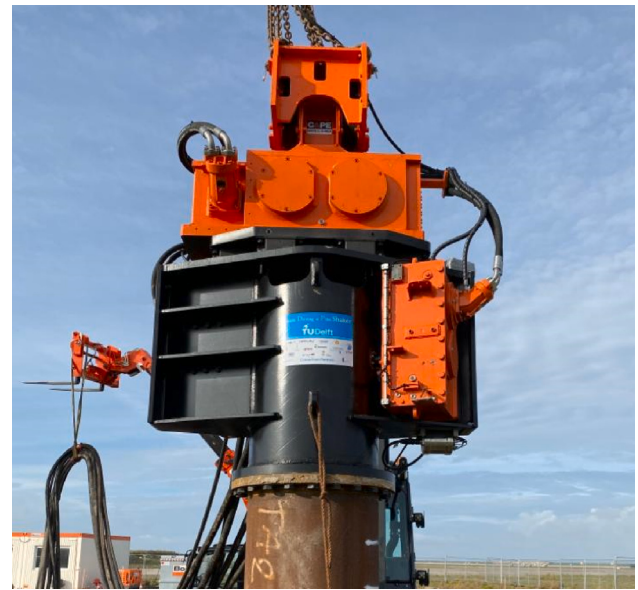
Fig. 1. The medium-scale GDP shaker connected to a pile via a bolted flange connection.
