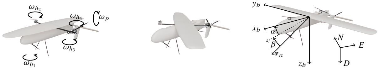
(a) VSQP at \Lambda = 0^\circ , in quad-mode configuration, with the propellers' rotation conventions used.
