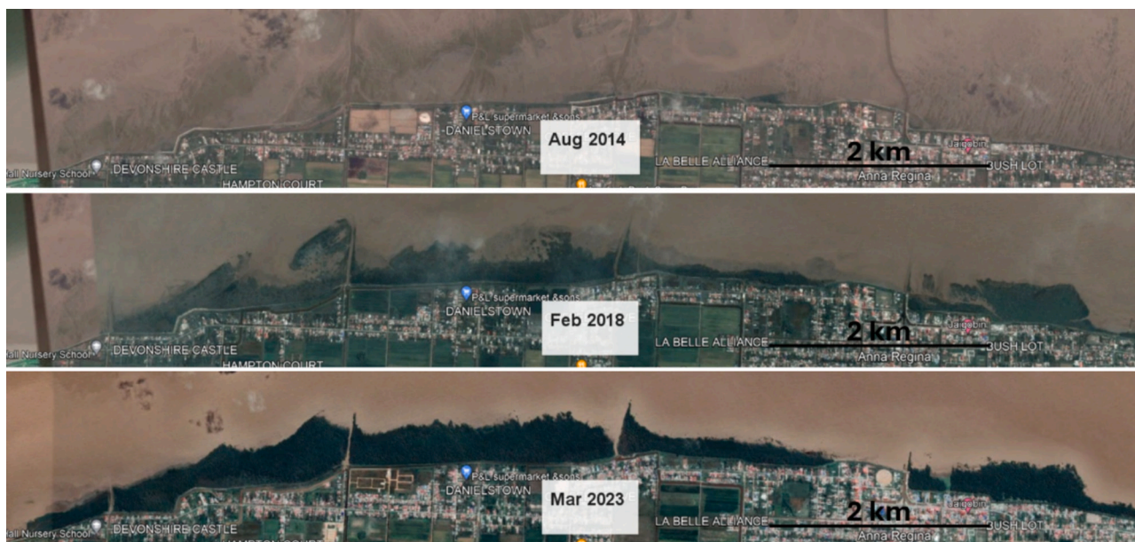
Fig. 6. Development of green-grey coastal defence infrastructure around Anna Regina (Google Earth satellite images). (For interpretation of the references to colour in this figure legend, the reader is referred to the web version of this article.)
