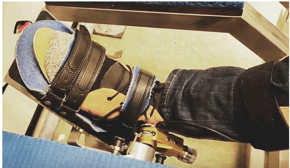
Figure 3. An example of how a patient was set up at the ankle manipulator for the measurement of the combined Ankle + Hermes PF torque. In this example, Hermes was used on the left leg.
