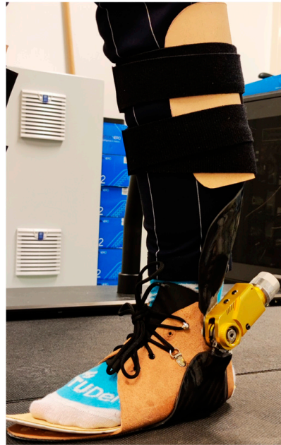
Figure 2. A photo of a participant wearing Hermes on the left leg. Hermes is composed by calf and foot parts made of prepreg carbon fiber and fabricated by an experienced orthotist.
