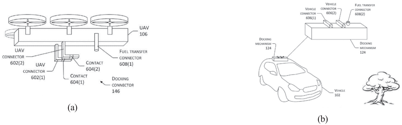
Fig. 3. Illustration of drone charging concept by Amazon (Raj, 2018).
