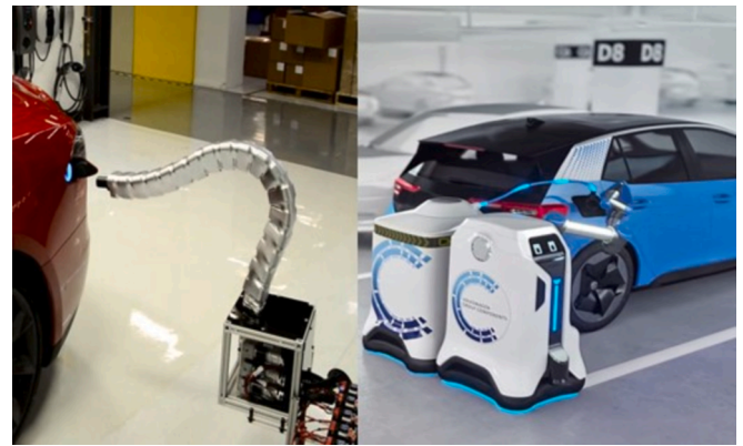
Fig. 8. Mobile charging bots (Hirz et al., 2021).
