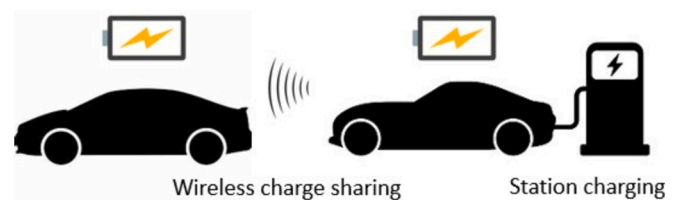
Fig. 13. Charging from fixed chargers and sharing charger with other vehicles proposed in (Mou et al., 2018).
