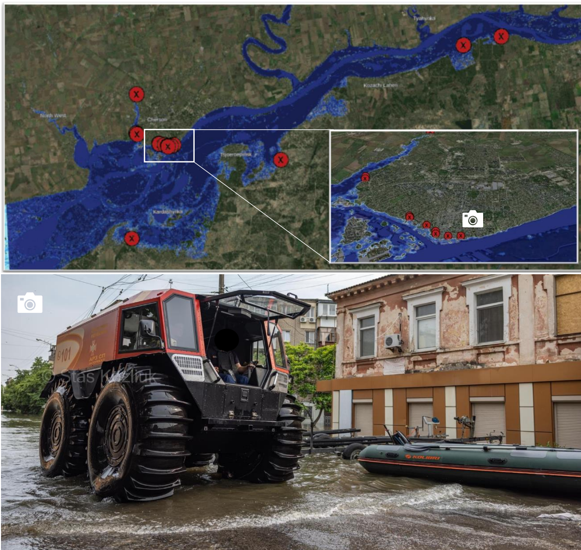
Figure 3: Overview of picture geolocations provided by a local environmental engineer from Kherson, showing the accuracy of the flood model in relation to observed flooding extents and an example of one of the pictures with geolocations.
