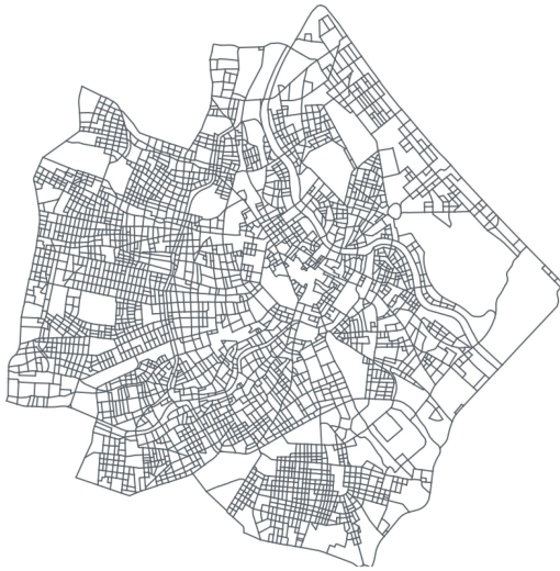
FIGURE 2. Constrained airspace structure extracted from the street network of the city centre of Vienna.
