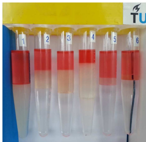
Fig. 1 Phase behaviour of IOS and n -hexadecane with the glass tube salinity scan method. Salinity (NaCl) varies from left to right (1.0 to 6.0 wt%) in the surfactant solution
