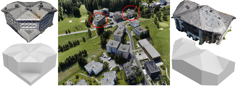
Figure 3.11: Reconstruction from aerial point clouds. In these point clouds, the vertical walls can be extracted from the point clouds and directly used in reconstruction, and thus the vertical plane inference step was skipped. The dataset is obtained from [31].
