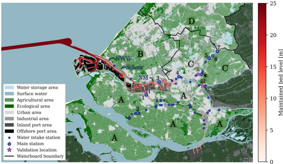
Figure 5.2: Overview of the land-based and water-based functions in the RMD , including the design of maintained bed levels of the Port of Rotterdam and the water intake stations. Labelled water boards: (A) Hollandse Delta; (B) Delfland; (C) Schieland & Krimpenerwaard; and (D) Rijnland. The numbered water intake stations correspond with Table 5.1. The water intake station labelled with a * represents the water intake stations upstream of the Hollandsche IJssel (5, 6, and 7). The lowercase, Roman numerals represent locations of data validation presented in Figure 5.4: (i) Spijkenisse-burg, (ii) Krimpen a/d IJssel, and (iii) Kinderdijk.
