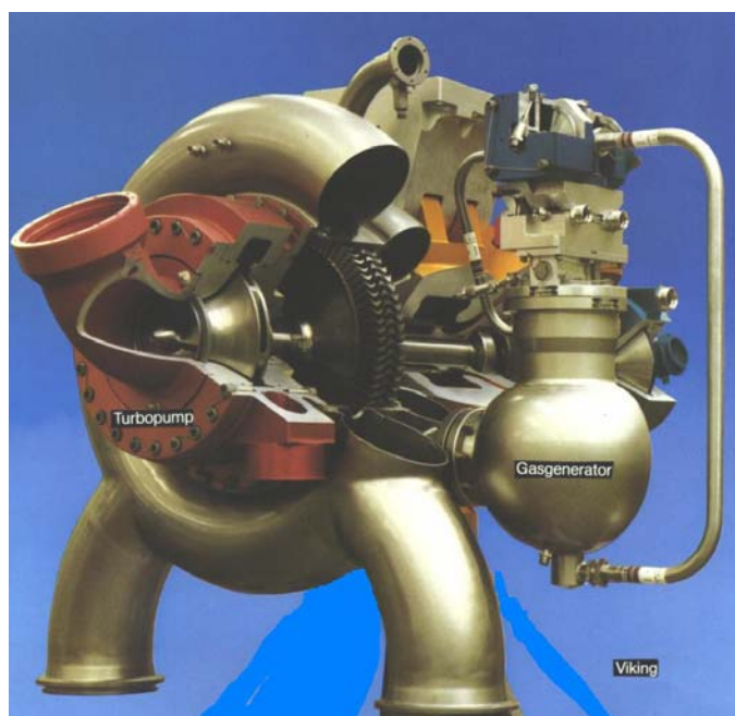
Figure 20: Viking V turbo-pump with gas generator (courtesy Snecma)
