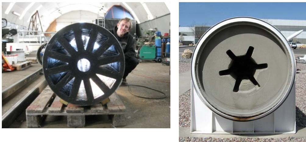
Figure 16: Examples of internal burning grains (left wagon wheel, right cylindrical with fins)
