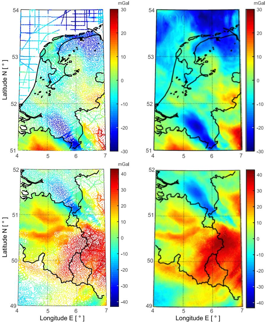
**Fig. 2.** Gravity anomalies in two  $3^\circ \times 3^\circ$  areas in the Netherlands: the measured surface gravity anomalies (left) and the  $2'' \times 2''$  “topography-implied and measurement-adjusted gravity anomalies” (right). The selected flat and rough  $1^\circ \times 1^\circ$  test areas are located at the centre of the areas shown in the top and bottom rows, respectively.
