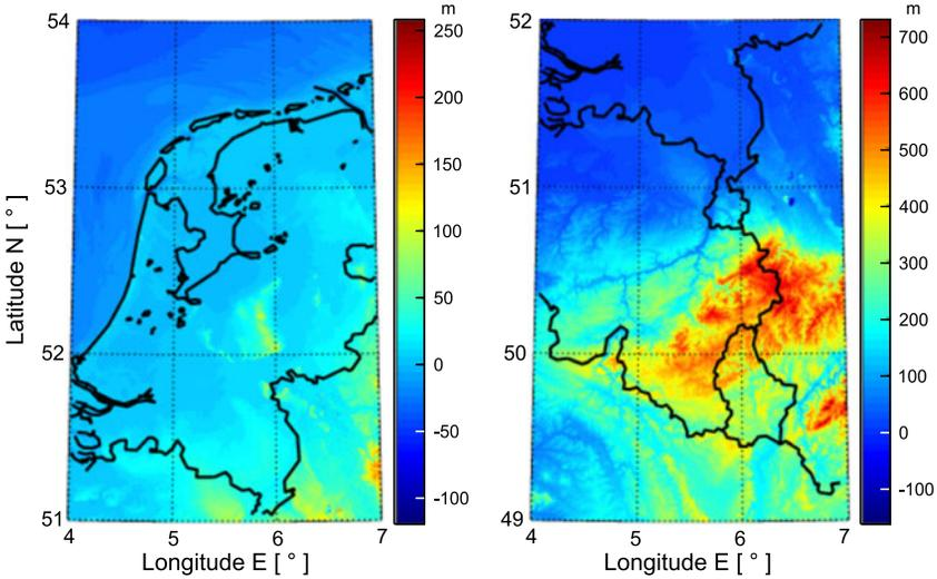
**Fig. 3.** Topography and bathymetry on a  $2'' \times 2''$  grid over two selected  $3^\circ \times 3^\circ$  areas in the Netherlands. The  $1^\circ \times 1^\circ$  test areas are located at the centre of the areas shown in the plots. The test area shown in the left panel is flat with little topography or bathymetry, whereas the one shown in the right panel is characterized by a rougher terrain, particularly in the south-eastern part with mountains up to 800 m.
