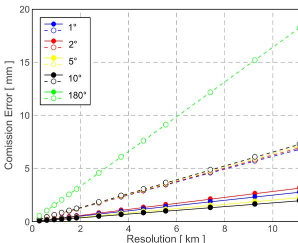
**Fig. 5.** Height anomaly commission error as a function of the data resolution for zero-mean white Gaussian noise of 1 mGal standard deviation in surface gravity anomalies when using the spherical Stokes integral (dashed lines) and the spheroidal Stokes integral (solid lines). Lines need to be scaled by  $x$  if the data noise standard deviation is  $x$  mGal.
