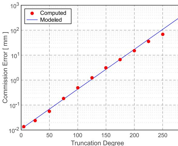
**Fig. 7.** Commission error of height anomalies (dots) for the global gravity field model GOCO05S as function of the truncation degree, computed along the southern border of the Netherlands (about 50°N latitude). For this latitude and geographic location, it can be well described by Eq. (42) (line).
