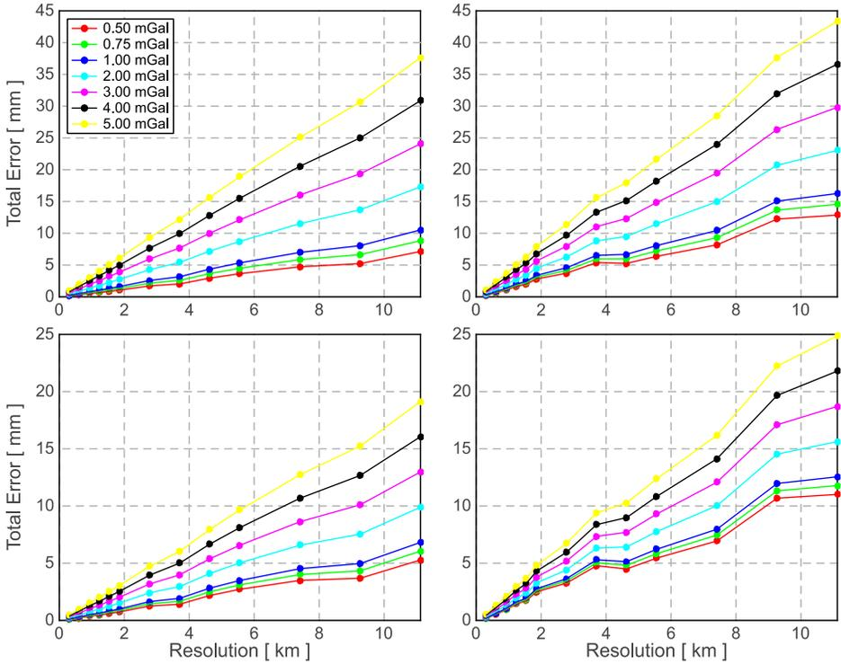
**Fig. 8.** Sum of commission and omission errors for the selected flat target area (top) and the rough target area (bottom) over the Netherlands for different noise standard deviations of the surface gravity anomaly data. The Stokes kernel (left column) and the spherical Stokes kernel (right column) are used when computing the commission error.
