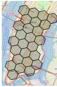
Figure 3.3: Hexagonal zone discretization of Manhattan core.
