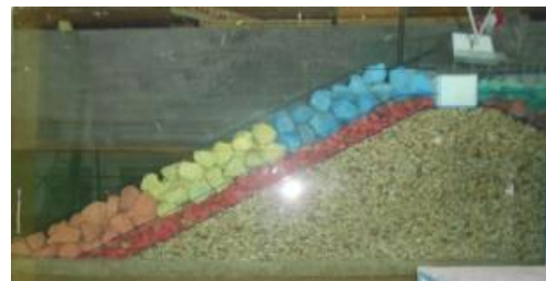
Figure 3. Model setup in LNEC flume.
