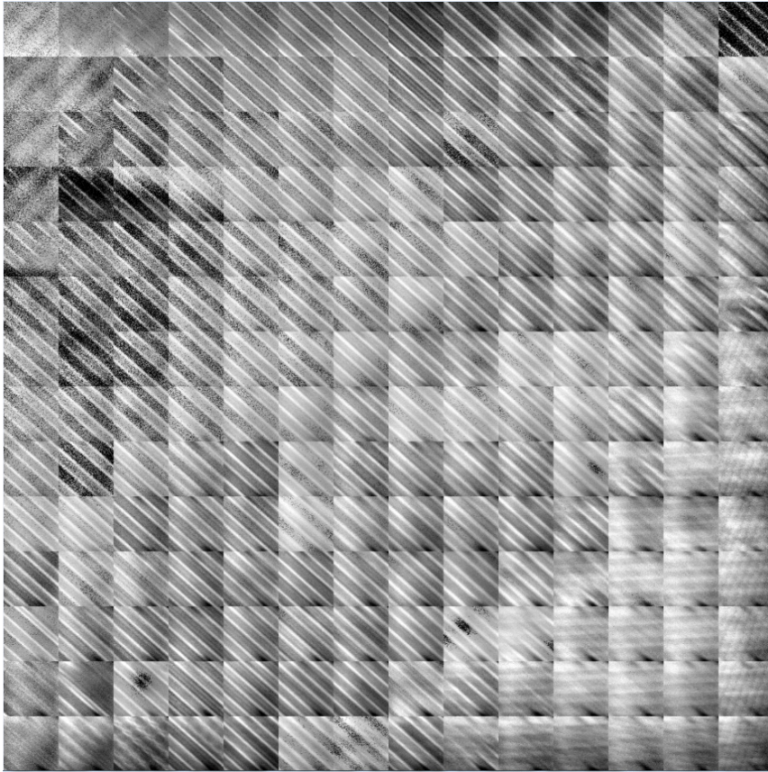
FIG 5. 18 A SE image map using calibration sample, with an FOV of 38\mu\text{m} and 2100 \times 2100 pixels. It is acquired using the INT lens, the HR lens and the UHR Lens, 0.765, 1.88 and 5.387, respectively, the retarding lens 9800V and working distance 2 mm. The current of each beam-let is 30pA. The SE beams' grid image is shown in FIG 5. 15(b).
