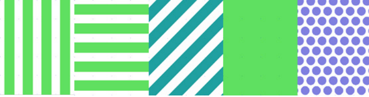
FIG 5. 14 Patterns in the calibration sample; the color part is electron transparent area, and the white is tungsten. Lines: 0.5\text{ }\mu\text{m} wide, 1\text{ }\mu\text{m} pitch; holes: 0.4\text{ }\mu\text{m} diameter, 0.6\text{ }\mu\text{m} pitch.
