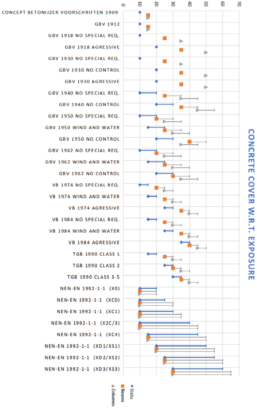
Figure A1.3: graphical presentation of concrete cover in relation to exposure
