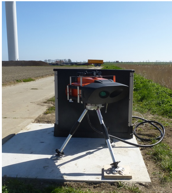
(b) Nacelle based LiDAR calibration facility
