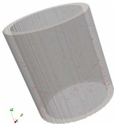
Figure 11: Crack pattern under low-restraint condition.
