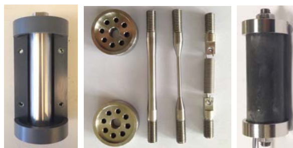
Figure 1: PVC mould and three types of restraints.
