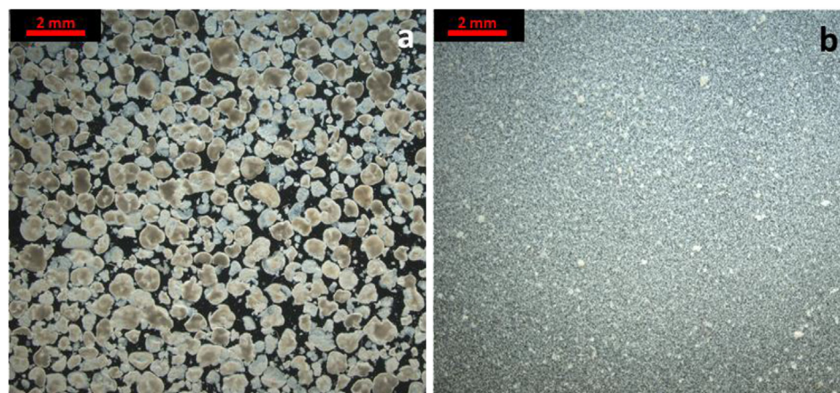
Fig. 5. A comparison between granules treated with sodium bicarbonate to extract ALE fraction (a) and acetic acid at 95 °C to solubilise the acid soluble EPS (b). Scale bar indicates 2 mm.
