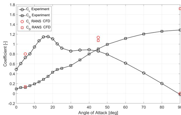
**Figure 4- Dynarig lift and drag coefficient curves**
