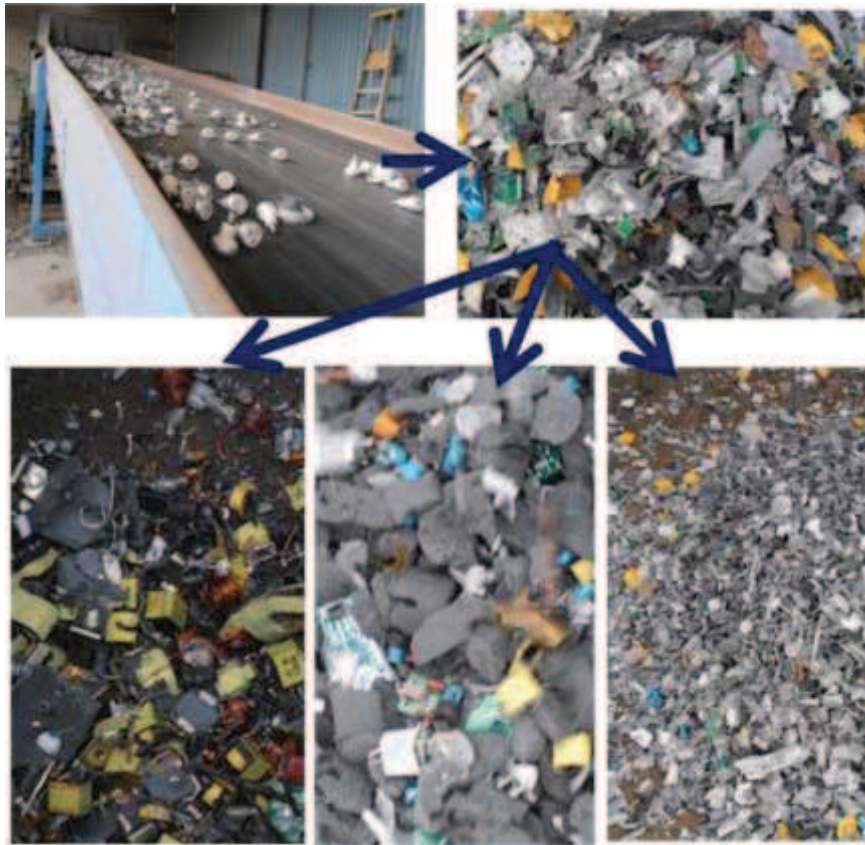
Figure 3. LED lamps and material fractions from large scale shredding of LED lamps [5].
