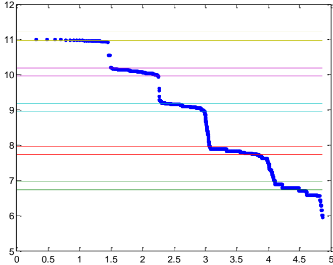
Figure 3.5: Sizes of particles found ( \log_2 of size on vertical axis), sorted from large to small ( \log_{10} of the index on horizontal axis). The screen sizes used for creating the input mixture are indicated as horizontal lines.
