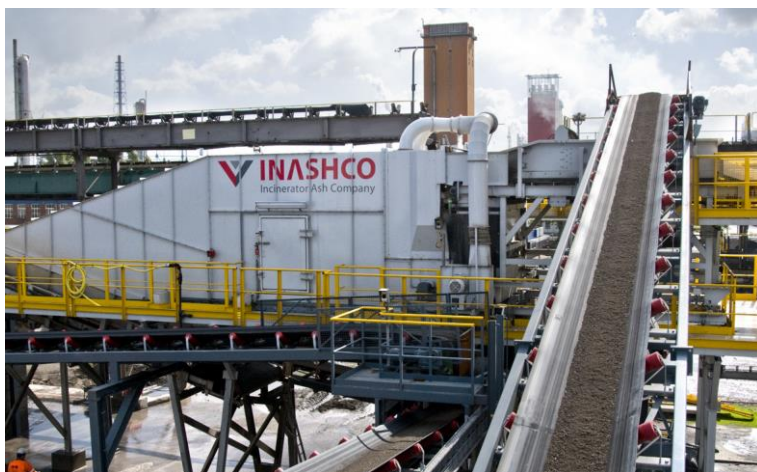
Figure 4.19: Industrial ADR operating at 120 t/h
