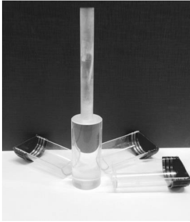
Figure 3.1: Equipment used: cups for handling parts of the mixture and a PMMA tube, inside volume 100 mm high, 10 mm diameter, 1 mm wall thickness.
