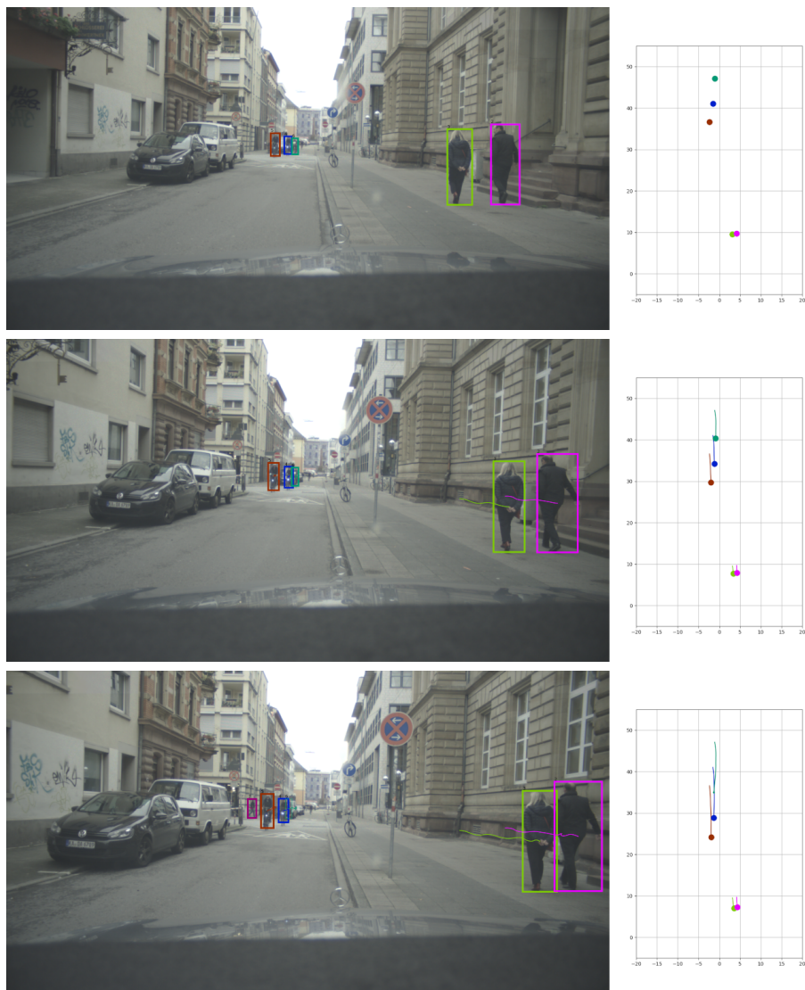
Figure 3.B.1: Additional qualitative results, showing all generated smoothed 3D positions in BEV next to each image. For each object, the trajectory history since the last keyframe is visualized both in the image and BEV. The scene depicts three cyclists at different distances coming toward the ego vehicle, as well as a couple walking on the sidewalk next to the street in front of the car. Best viewed in PDF format with zoom for optimal detail.
