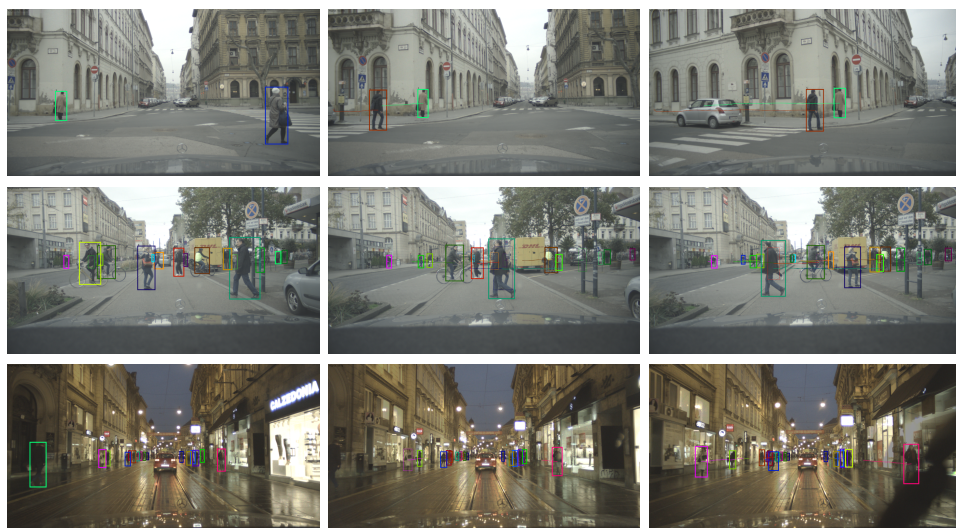
Figure 3.4: Qualitative results of the pseudo GT generation approach proposed in this thesis. A keyframe with the corresponding keyframe annotations is shown on the left and right, while the middle column presents the image in between the keyframes (1 s. apart from keyframes). Track IDs are shown by color-coded boxes. The history of each box in terms of the previous center positions is also shown. Best viewed when magnifying the PDF document. In the top row, a scene from Budapest, with few people during a high yaw-rate turn maneuver: it represents no problem for the proposed approach. The middle row shows a challenging scenario recorded in Karlsruhe, with multiple persons being partly and heavily occluded. Note how the trajectories for the persons are reliably generated also during occlusion (e.g., orange box in the center). Lastly, a challenging scene is shown in the bottom row, recorded at nighttime during rainfall in Zagreb. Here an error in the generated pseudo ground-truth can be observed. An ID-switch happens for the two persons on the left (red box with id 5, brown box with id 17), after being occluded by the crossing pedestrian (blue box id 4).
