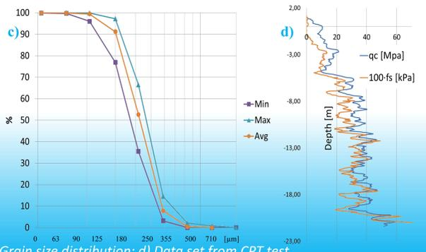
a) Qualitative description of a Flowslide; b) Picture of a typical suction dredger employed in sand quarries below ground water level in Belgium; c) Grain size distribution; d) Data set from CPT test
