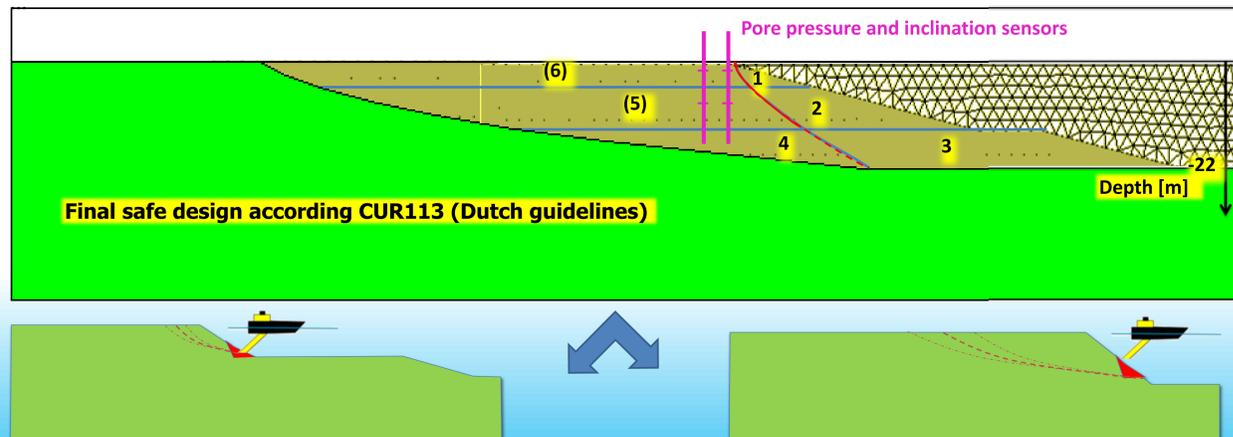
Transition from 'actual geometry' to 'real scale test geometry' to 'final geometry'. The range of expected failure mechanisms is visualized at two depths. Failure is expected to be triggered by achieving a fast rate of excavation (loading) on a steep slope.
