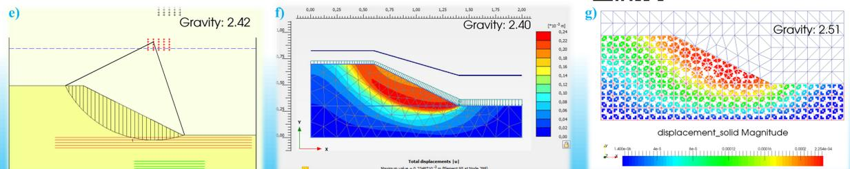
e) Bishop's slice method for slope stability analysis; f) Plaxis2D (FEM) simulation with quasistatic loading; g) Anura3D (MPM) simulation with quasistatic loading.
