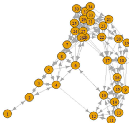
Figure 9. Storage plant of Fig. 6 as a weighted directed graph with active safety barriers in place.
